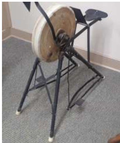
Grinding wheel used to sharpen axes and other tools on the farm or railroad.
